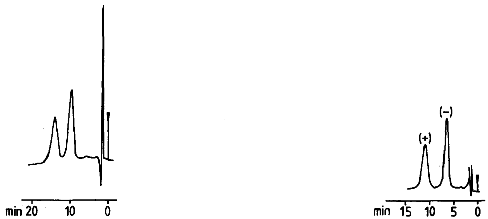
Fig. 9. Resolution of racemic pentazocine. Conditions as in Fig. 8. The enantiomers are not available in pure form.
